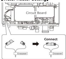
Connect the connector marked "Crossover" inside of the Water Heater.
