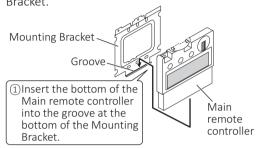
②Push in the 2 hooks on top of the Main remote controller completely.
