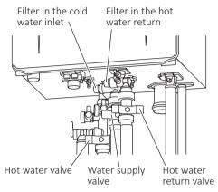
2) With a bucket ready, remove the water drain valves.
