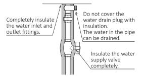
**NOTE** In order for the freeze prevention heaters to operate, the Water Heater must connect the electrical power at all times.
