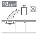
• Install in a location where the exhaust gas flow will not be affected by fans or range hoods.
