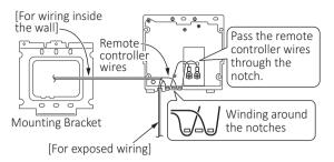
6. Attach the Remote Controller to the Mounting Bracket.
