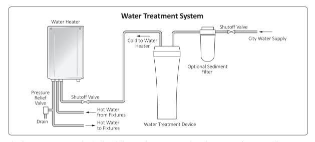
The illustration is an example. Check with the actual Water Heater about the position of piping, and form.
