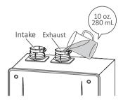
If the vent pipe has already been installed: After installing the condensate drain pipe, make sure that the area around the Water Heater is well ventilated; open a window or a door if necessary. Then, operate the Water Heater and verify that condensate is coming out of the condensate drain pipe.
