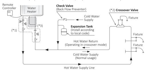
(\*1) Noritz America stocks the "Isolation Valve" (Service Valve Kit) for easy water line installation. The Isolation Valve (Service Valve Kit) is necessary for flushing the Heat Exchanger.
