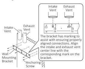
2. Hang the Water Heater on the Wall Mounting Bracket.
