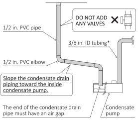
\* Install tubing according to pump manufacturer's instructions.
