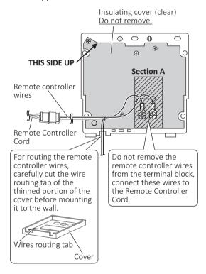
Check the terminal is covered with Section A
