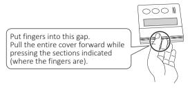
If it does not come off, insert a flat head driver into the notch at the bottom of the cover and slightly twist it to remove.
